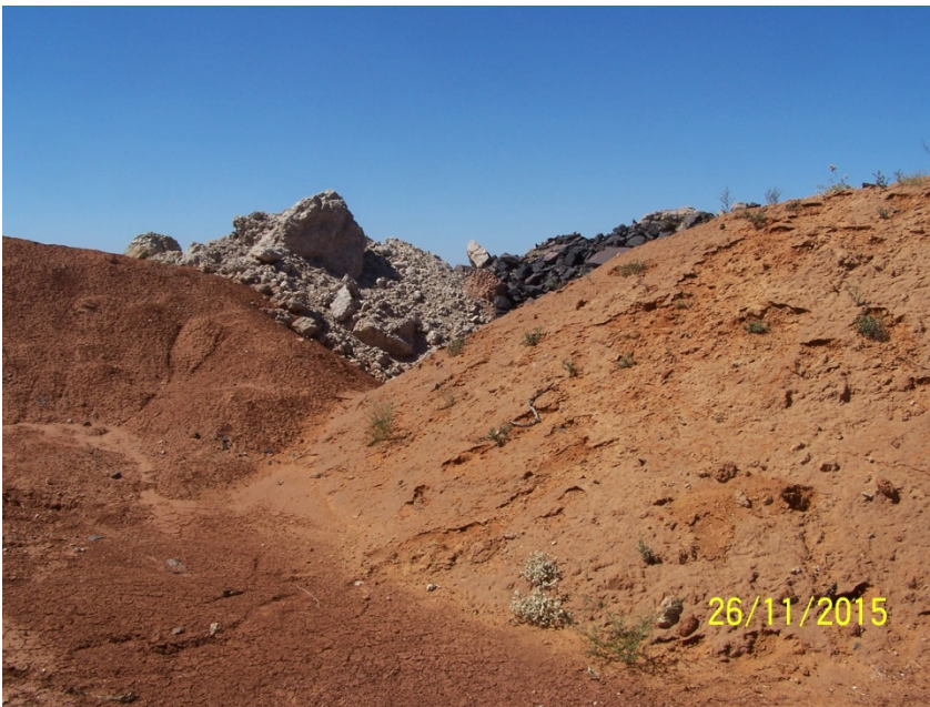
Figure B2: Dark reddish brown clay (right), conglomerate and black shale material (centre) and red Kalahari sands (left) on the Western dump
