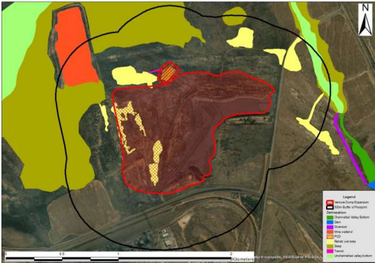
Figure 24. Map of the proposed Venture Dump extension in relation to delineated wetland habitat.
