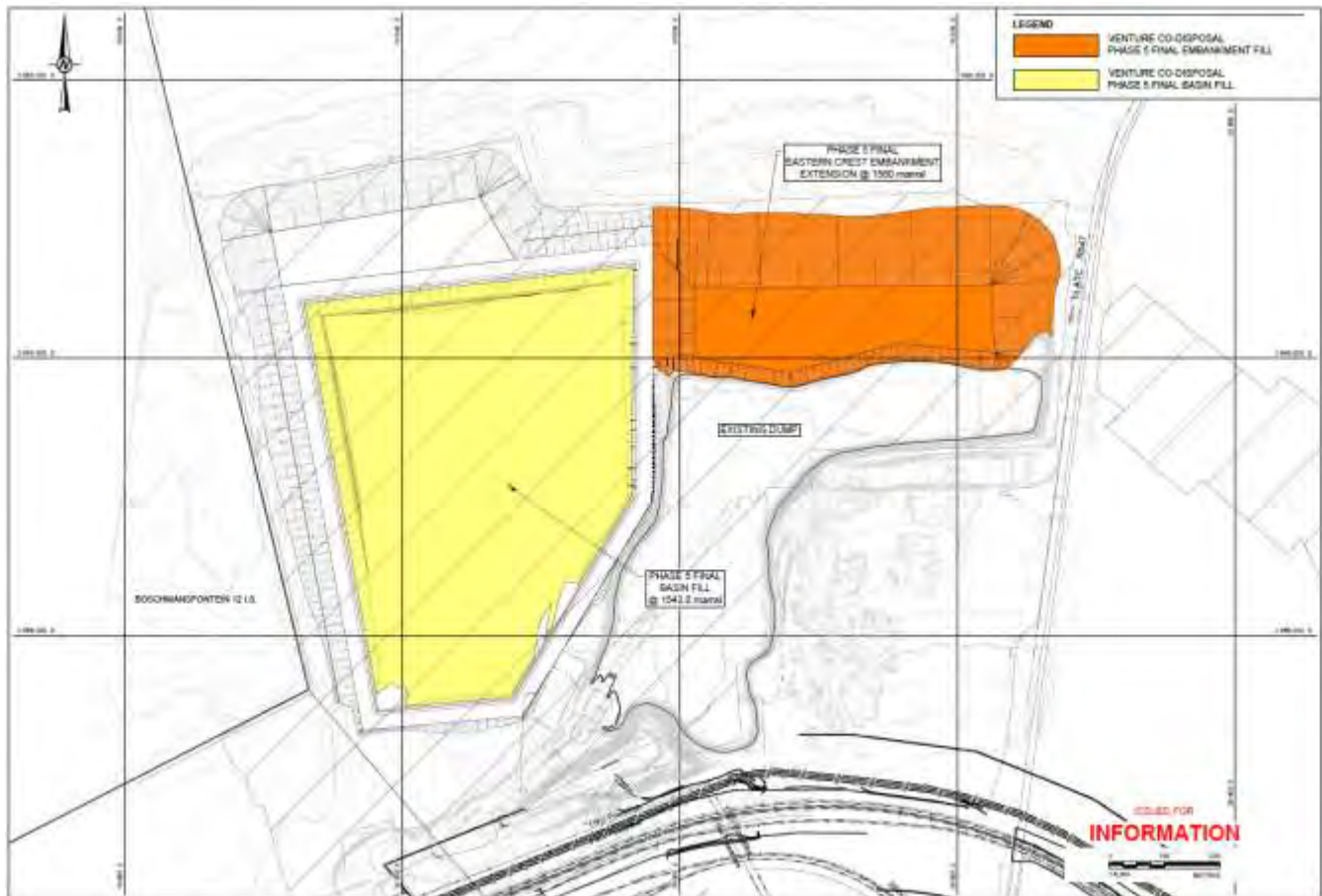
Figure 9: Phase 5 Final Layout - Venture Co-disposal Facility.
