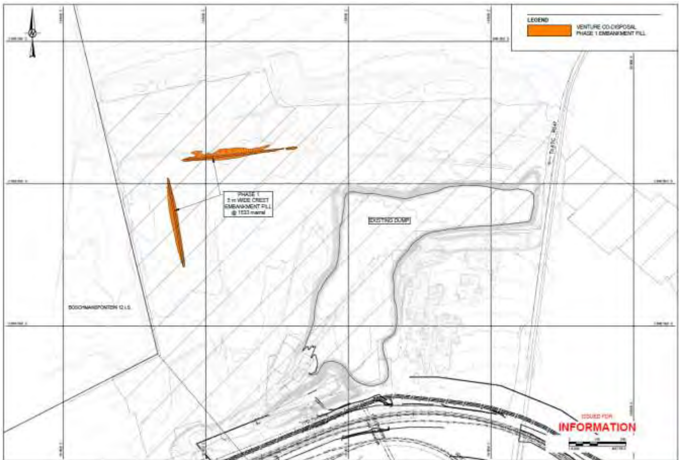
Figure 4: Phase 1 Layout - Venture Co-disposal Facility.
