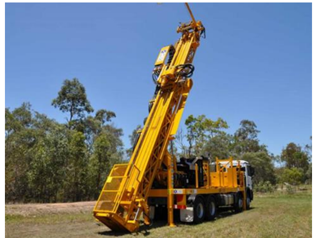
Figure 2: Typical core drilling rig
