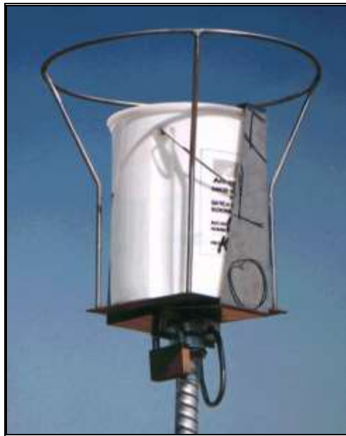
Figure 1: Single bucket monitoring unit, showing sampling bucket with bird ring and security clamp
