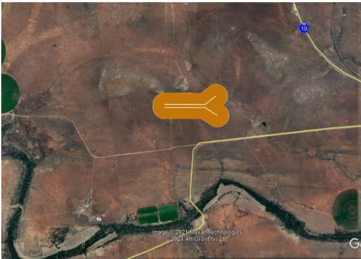
Figure 3b. The two incoming and outgoing powerlines with a 300m corridor each from the proposed 400kV substation to the existing 400kV Eskom powerline.
