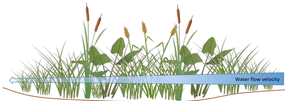
Figure 8: Wetland plants play a crucial role in slowing water flow, while allowing infiltration of water into the soils below.
