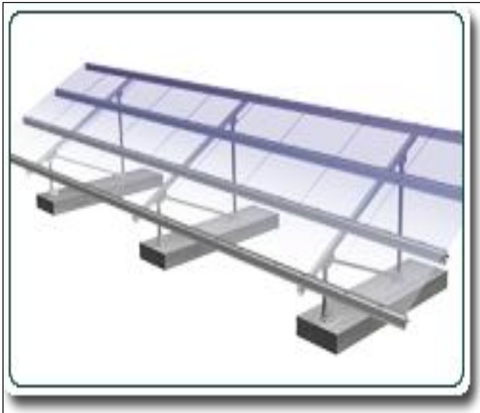
Figure 3. Solar panel (non rotating) placed on strip footings
