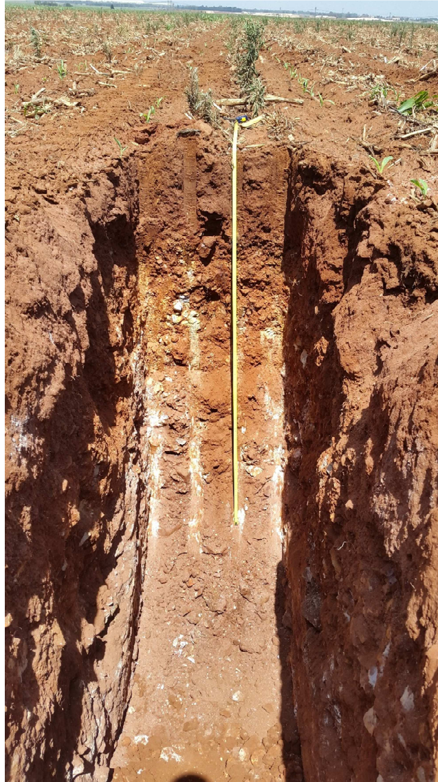
Figure 5: Typical profile of the dolomite at test pit PV42
