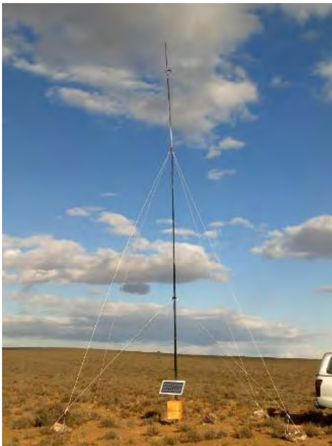
Figure 6: Short mast monitoring system
