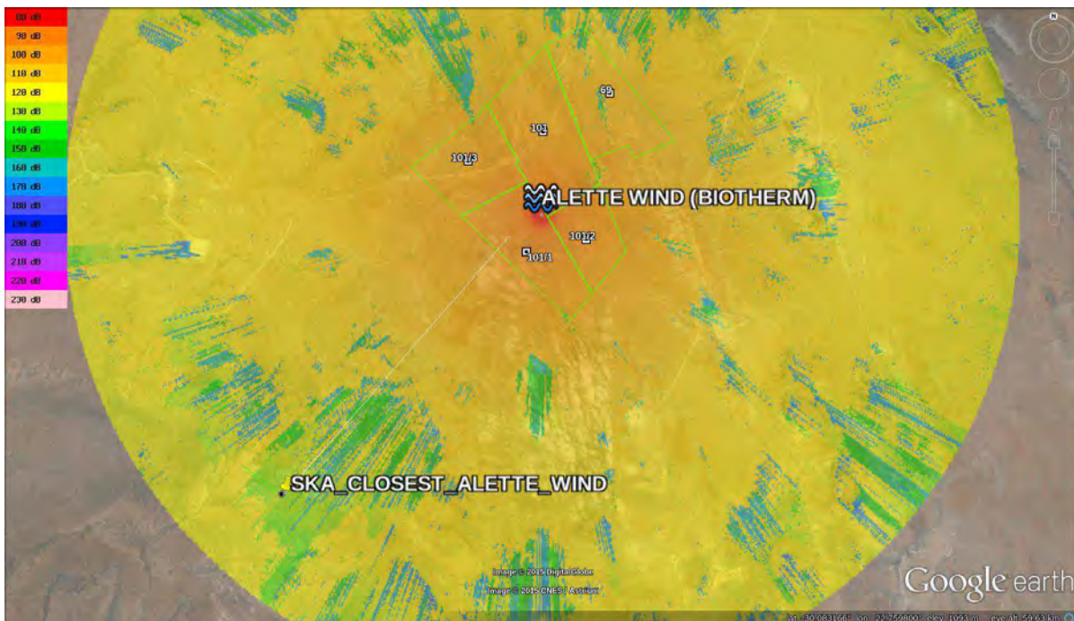
Figure 7: Attenuation map for f=1000MHz from Aletta Wind to the closest SKA telescope.
