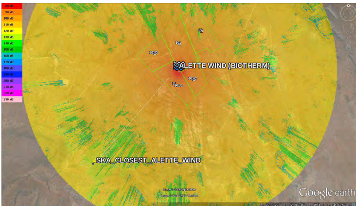
Figure 5: Attenuation map for f=500MHz from Aletta Wind to the closest SKA telescope.
