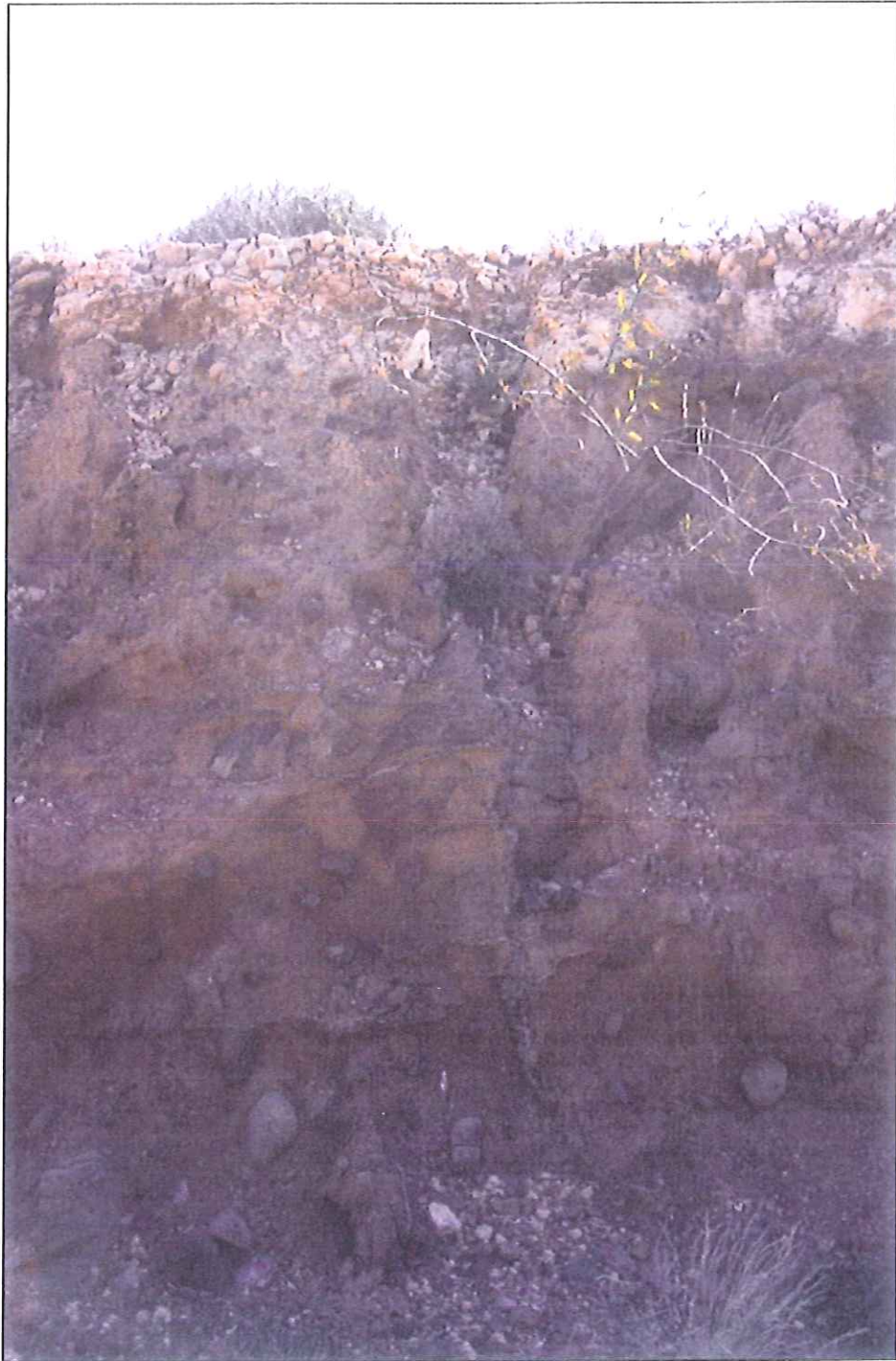
Completely weathered much younger Dwyka tillite with poorly sorted angular to sub-rounded clasts of various origins.
