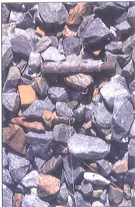
Dumo rock, used as railway ballast; rich in sulphides, hence corrosion of metal objects that have been exposed to this material for some time.
