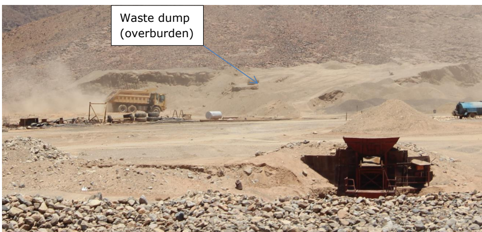
Plate 6: Dump truck in front of waste dump in background The dump truck is 4.3m in height. The dump should be anything between 7-8m high. (Naledzi)
