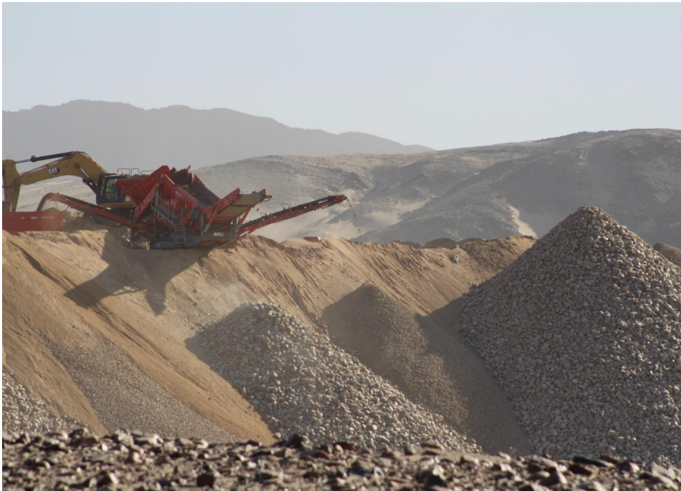
Plate 4: Example of Infield Screen tipping out coarse and fine tailings Photo taken at Reuning (Naledzi)
