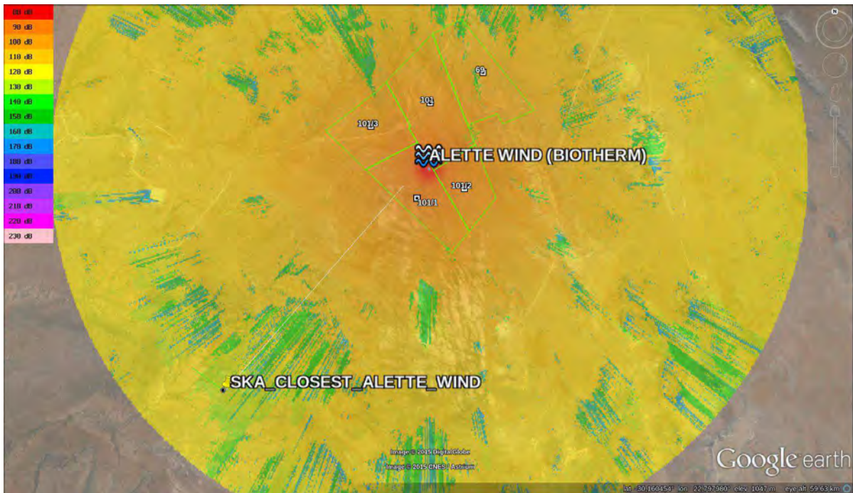
Figure 6: Attenuation map for f=700MHz from Aletta Wind to the closest SKA telescope.
