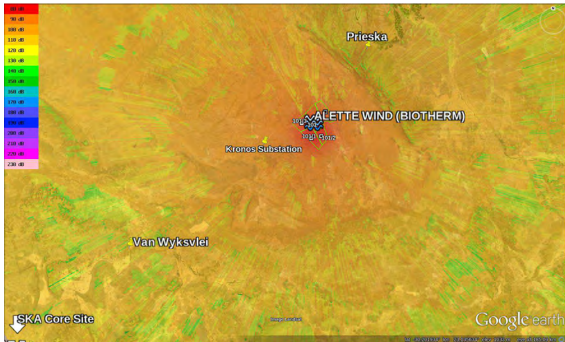
Figure 11: Attenuation map for f=100MHz from Aletta Wind to the SKA core.
