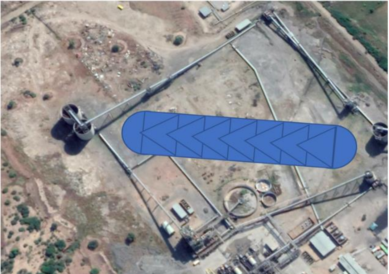
Figure 3: Conceptual design of the proposed product stockpile
