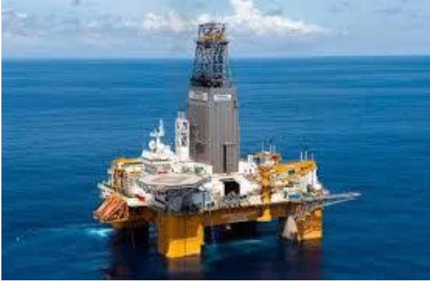
Figure 1-2 - Example of semi-submersible drilling vessel
