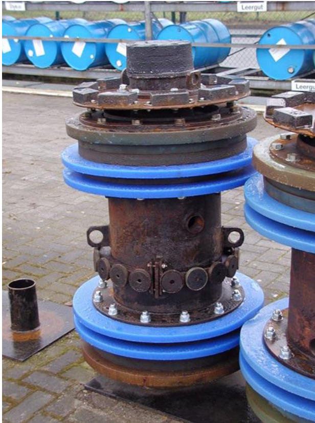
Figure 7-3 - Typical Pipeline Cleaning Pig (from https://en.wikipedia.org/wiki/File:NWO-MolchPlastik2.jpg )
