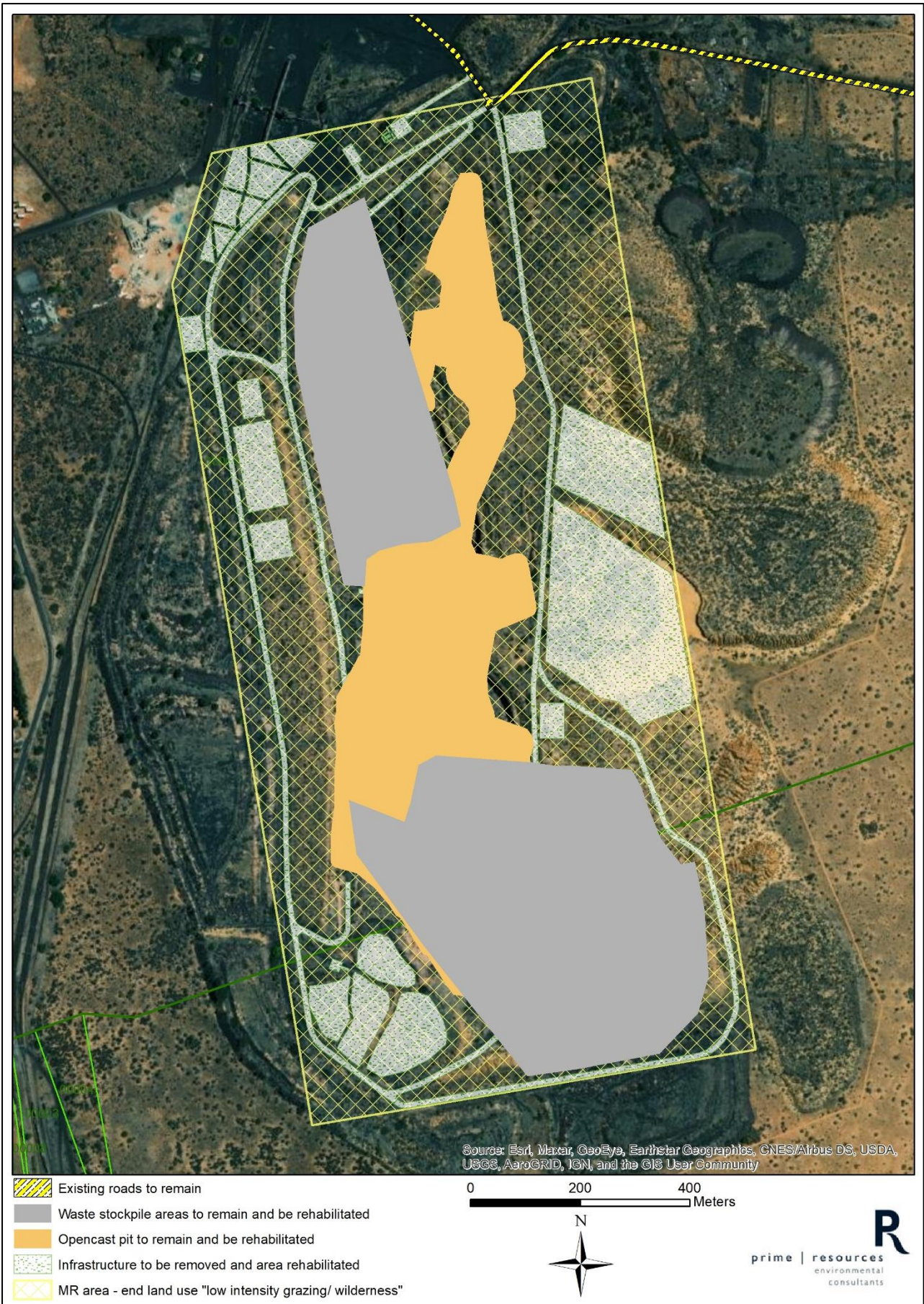
Figure 7: Infrastructure to remain post-closure and high-level final end land use plan for the THM area
