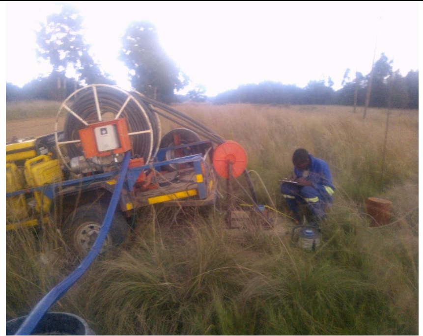
Data recording during pumping test
