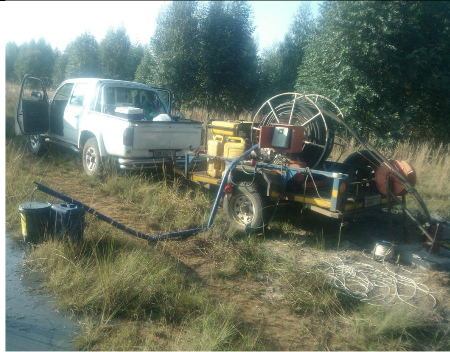
Calibration test using submersible pump
