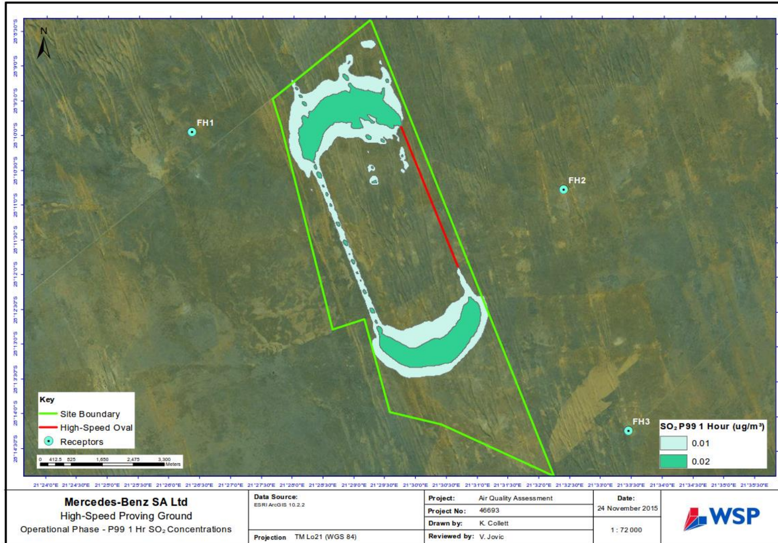
Figure 20: Predicted P99 hourly SO 2 concentrations associated with the operational phase of the Proposed High-Speed Proving Ground
