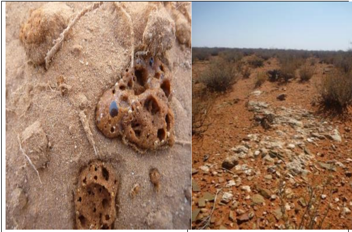
Figure 6: Photo left-Free lime in soil fizzes when reacted with 10% HCl, Photo right-Calcrete daylight in areas where the Coega soil form dominates
