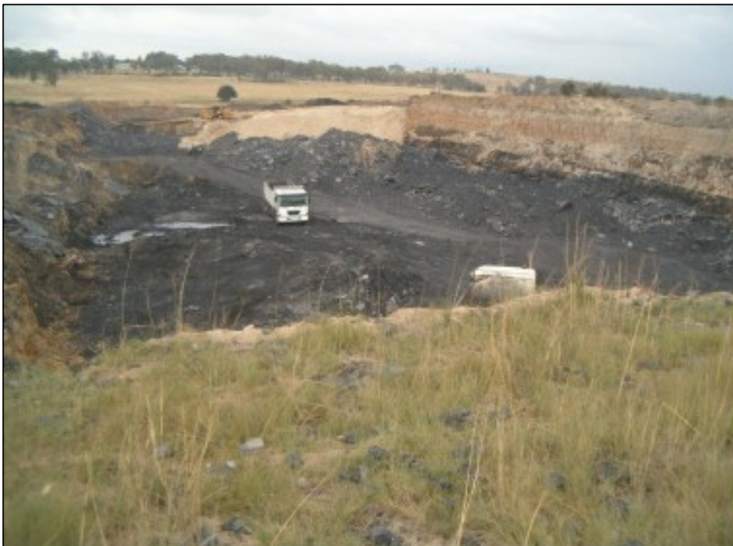
Figure 5: A typical box cut.
