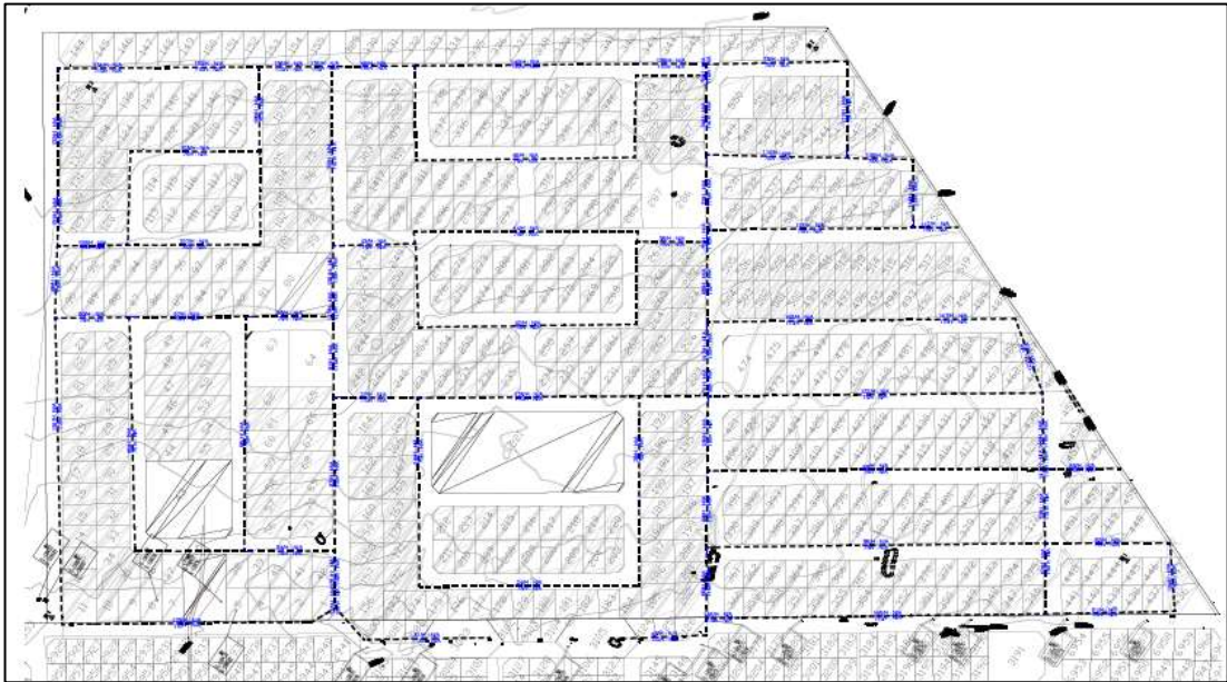
Figure 4: Proposed water network for Khalinkomo
