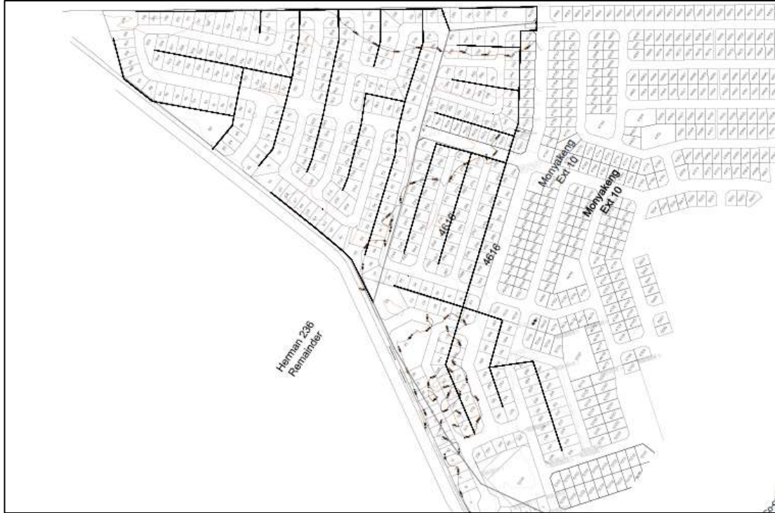
Figure 7: Proposed Sewer Network in Vergenoeg
