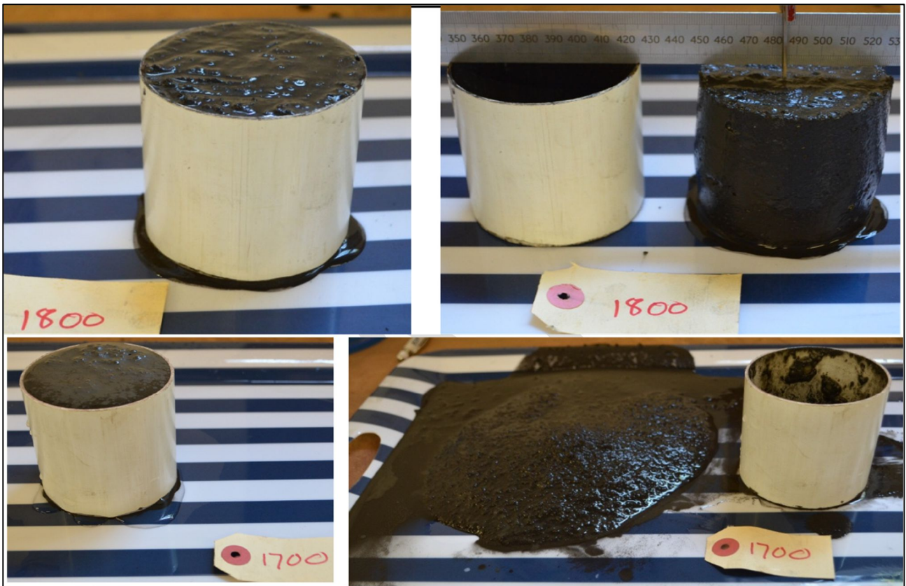
FIGURE 19: BOGER SLUMP TESTS
