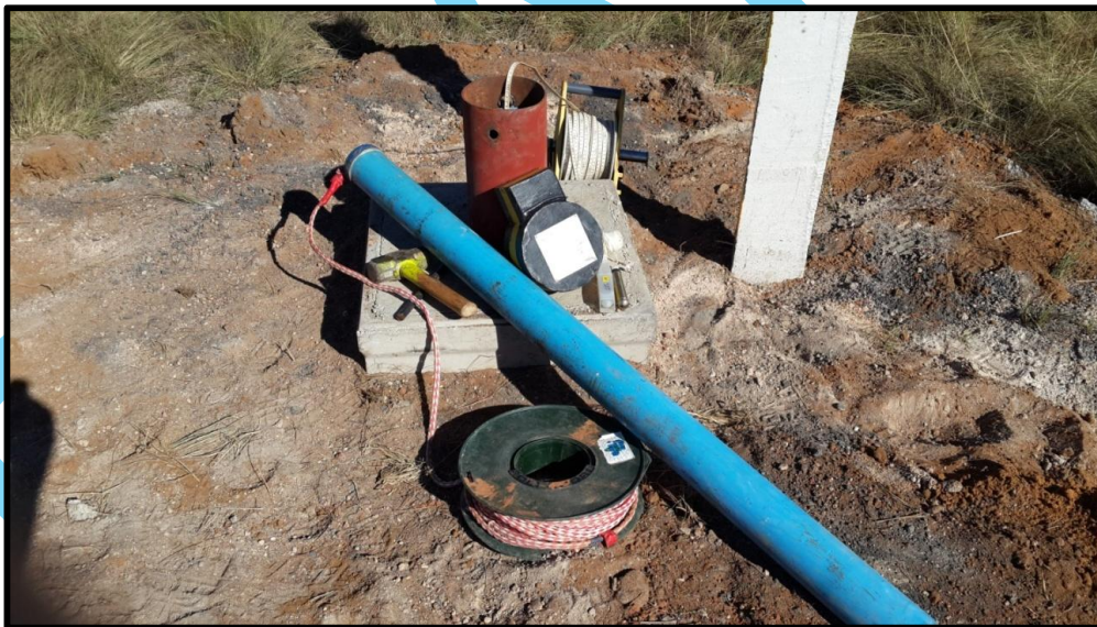
Figure 5 Slug test equipment setup
