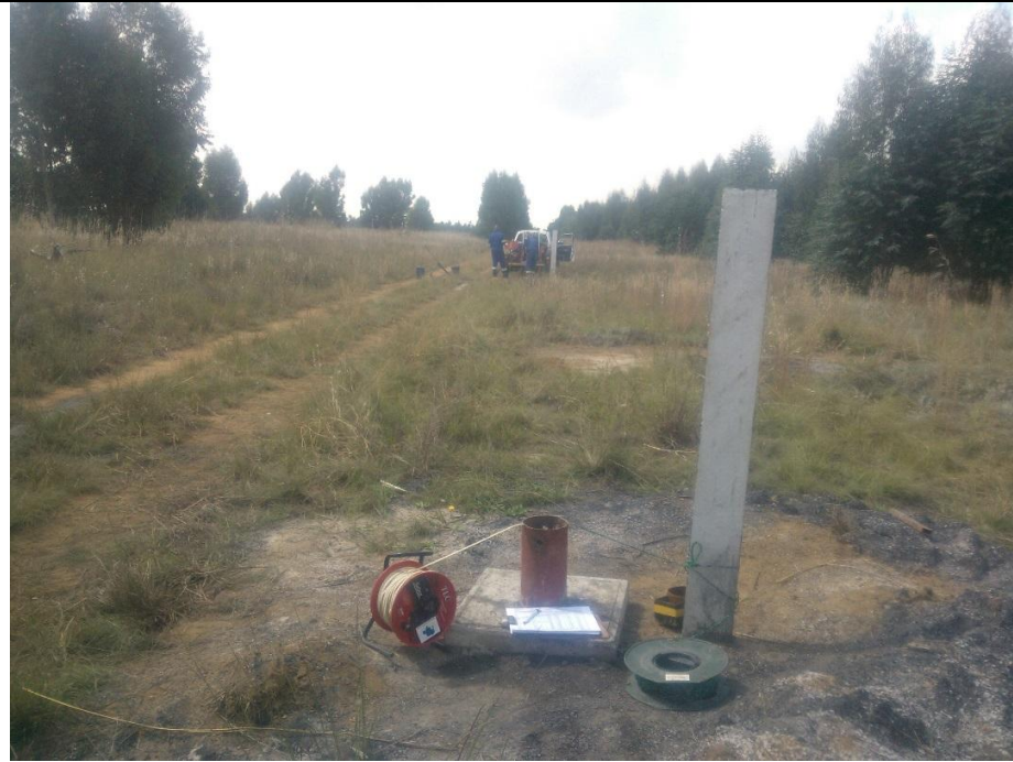
Water level measured in observation hole (while pumping the other hole)
