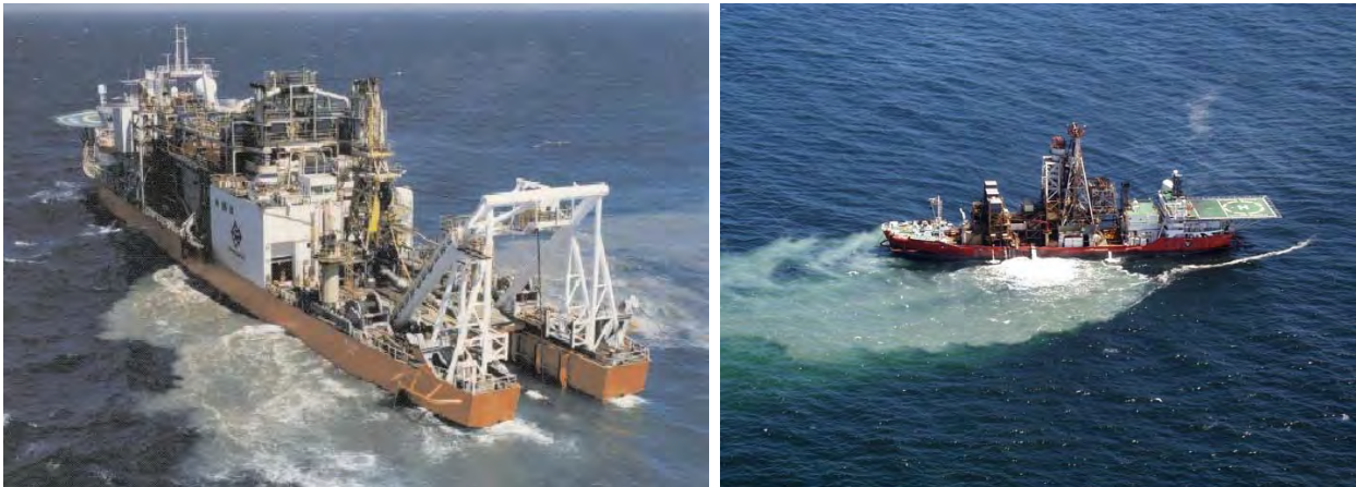
Figure 33: Typical crawler-vessel (left) and drillship (right) operating in the Atlantic 1 Mining Licence Area (Photos: De Beers Marine).
