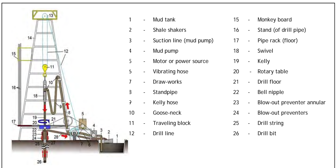
Figure 3: Flow path of the drilling fluid.
