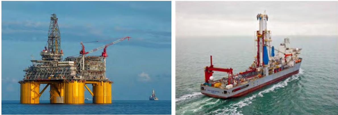
Figure 2: Typical semi-submersible drilling rig (left) and drilling vessel (right) (Source: Shell).
