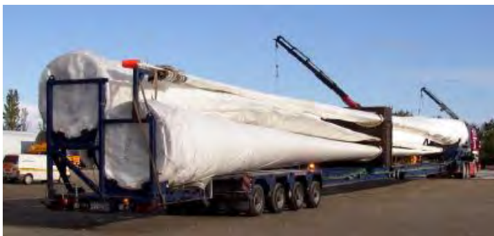
Figure 2: Example: 3 x 45m Blades on extendible trailers
