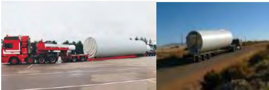
Figure 4: Transporting the Tower Sections
