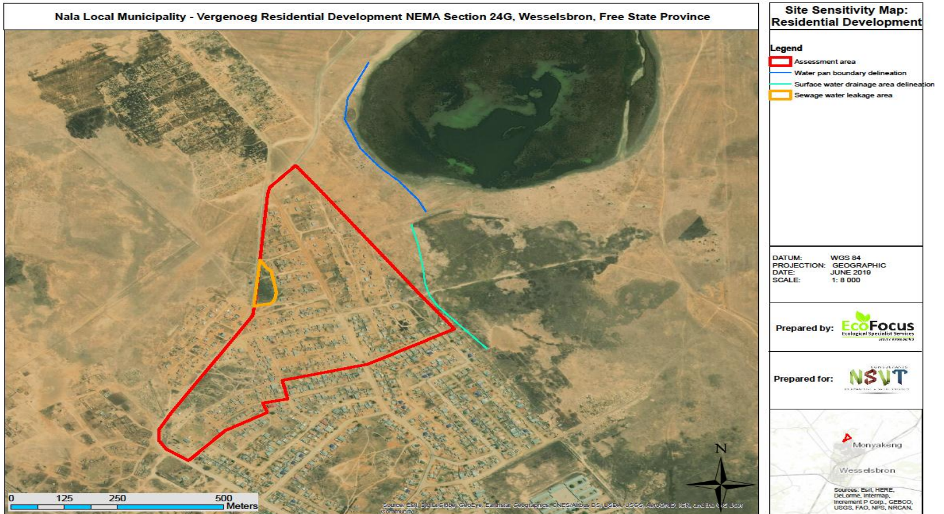
Figure 10: Site sensitivity map illustrating the delineation of the first water pan situated north-east of the assessment area as well as its associated surface water drainage area which flows from the south in a northerly direction past the assessment area, towards the pan (see A3 sized map in the Appendices)
