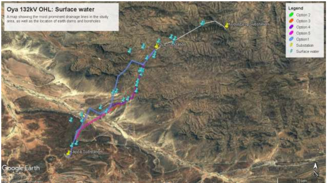
Figure 9: A map of the rivers and waterbodies (dams and boreholes) in the study area relative to the proposed corridor options.
