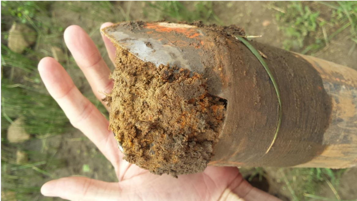
Figure 11. Sub-soil Sample drawn from within Natural Depression Wetland 1 showing Orange Mottling and Grey Reduced Soil Particles
