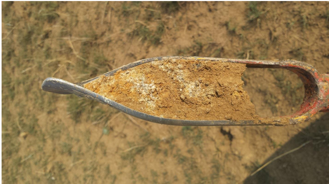
Figure 7. Soil Sample showing Orange Mottling and Carbonaceous Materials in the Soil Matrix
