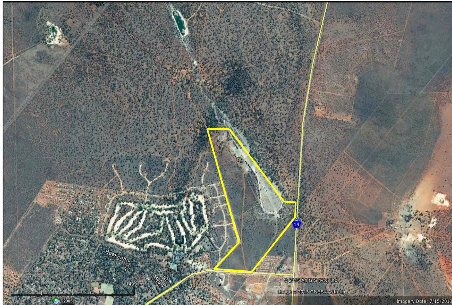
Fig. 2. Google earth© satellite image of the study area for the proposed Uitkoms housing development on the western side of the N14 and on the north-eastern outskirts of the town of Kathu, Northern Cape (yellow polygon). The prominent elongate grey area reflects near-surface calcretes along the Vlermuisleegte drainage line. This grey zone is of moderate palaeontological sensitivity.
