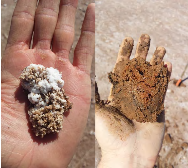
Figure 17. Salt Precipitation at the Surface (left) and Red Iron and Black Manganese Accumulations observed in the Sub-soils of a Saline Wetland
