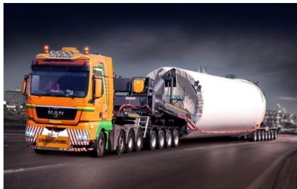
Figure 7.1 Example of Tower Sections Transport (Nootboom)
