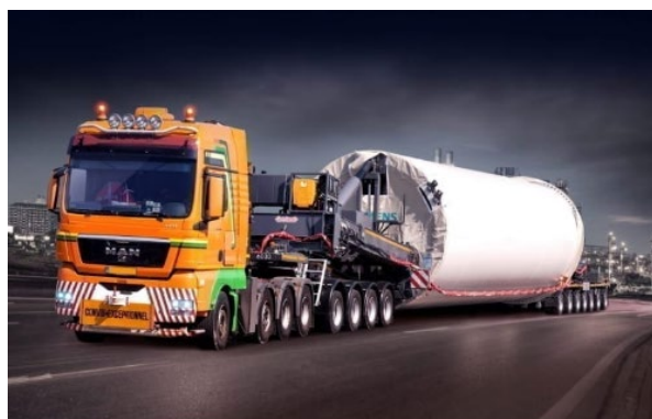
Figure 7.1 Example of Tower Sections Transport (Nootboom)
