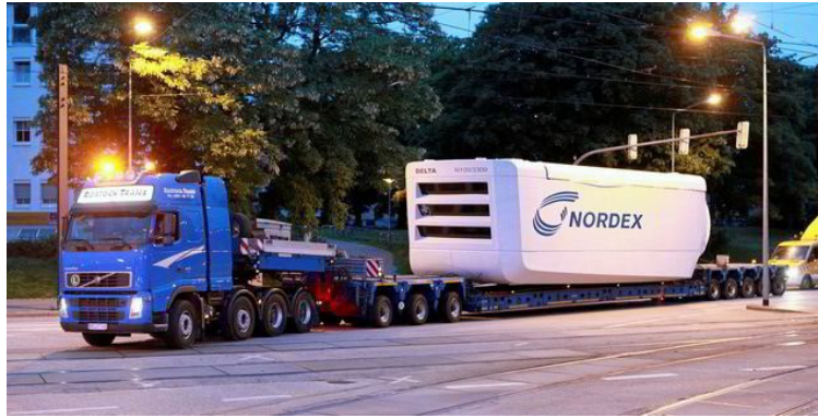
Figure 7.2 Example of Nacelle Transport ( Recharge News )
