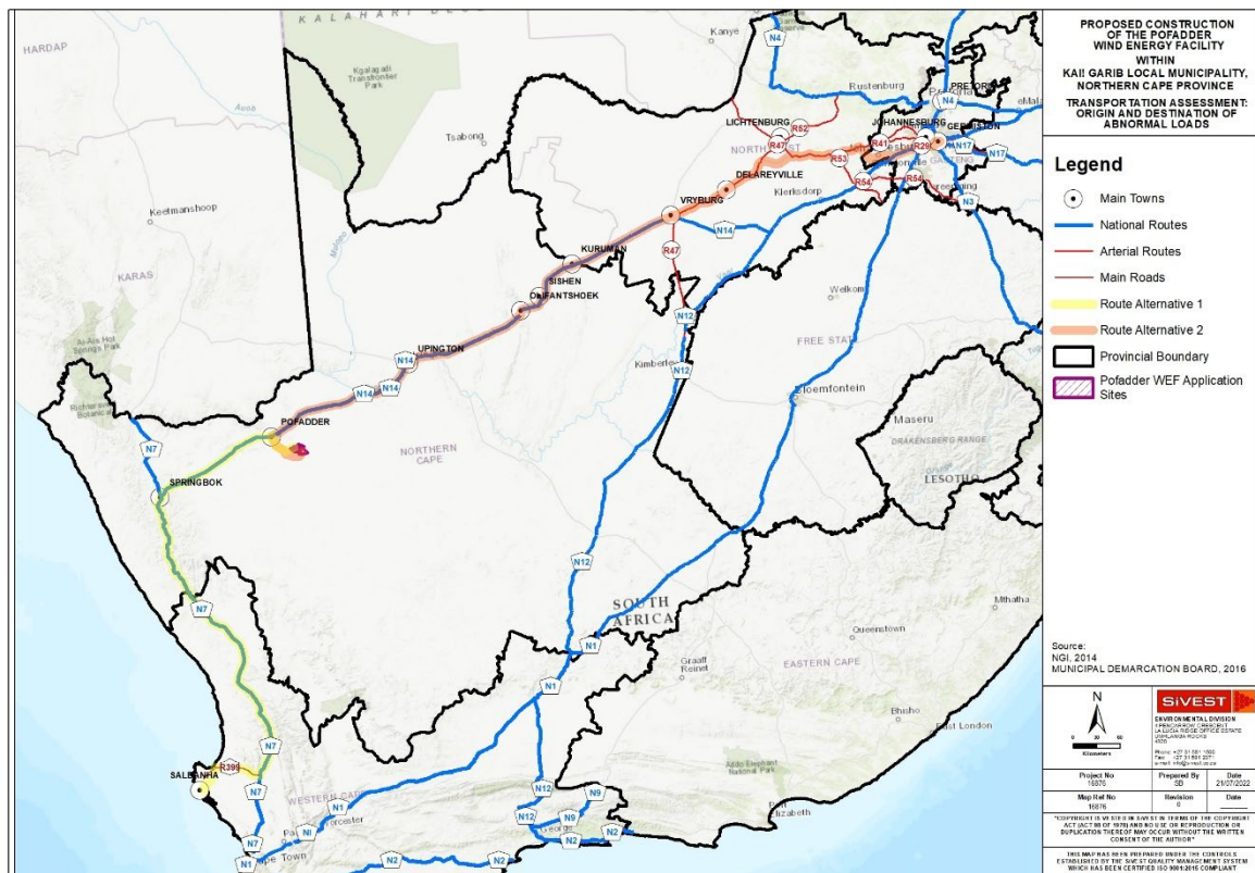
Figure 7.6 Normal & Abnormal Load Transport Route
