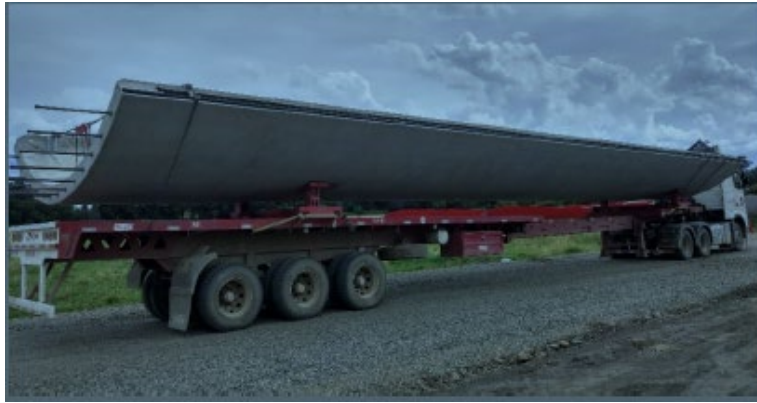
Figure 7.2 Example of Hybrid Tower Sections (Nordex)
