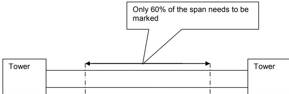
Figure 8: The section that needs to be marked
