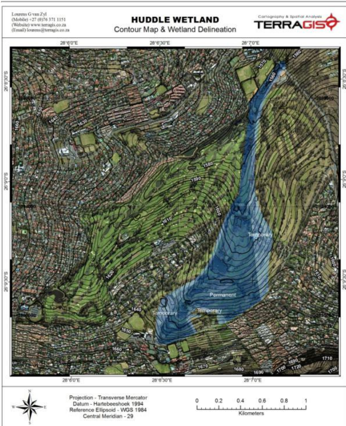
Figure 12. Satellite image with 2 m contours with a historic wetland delineation result superimposed on the image
