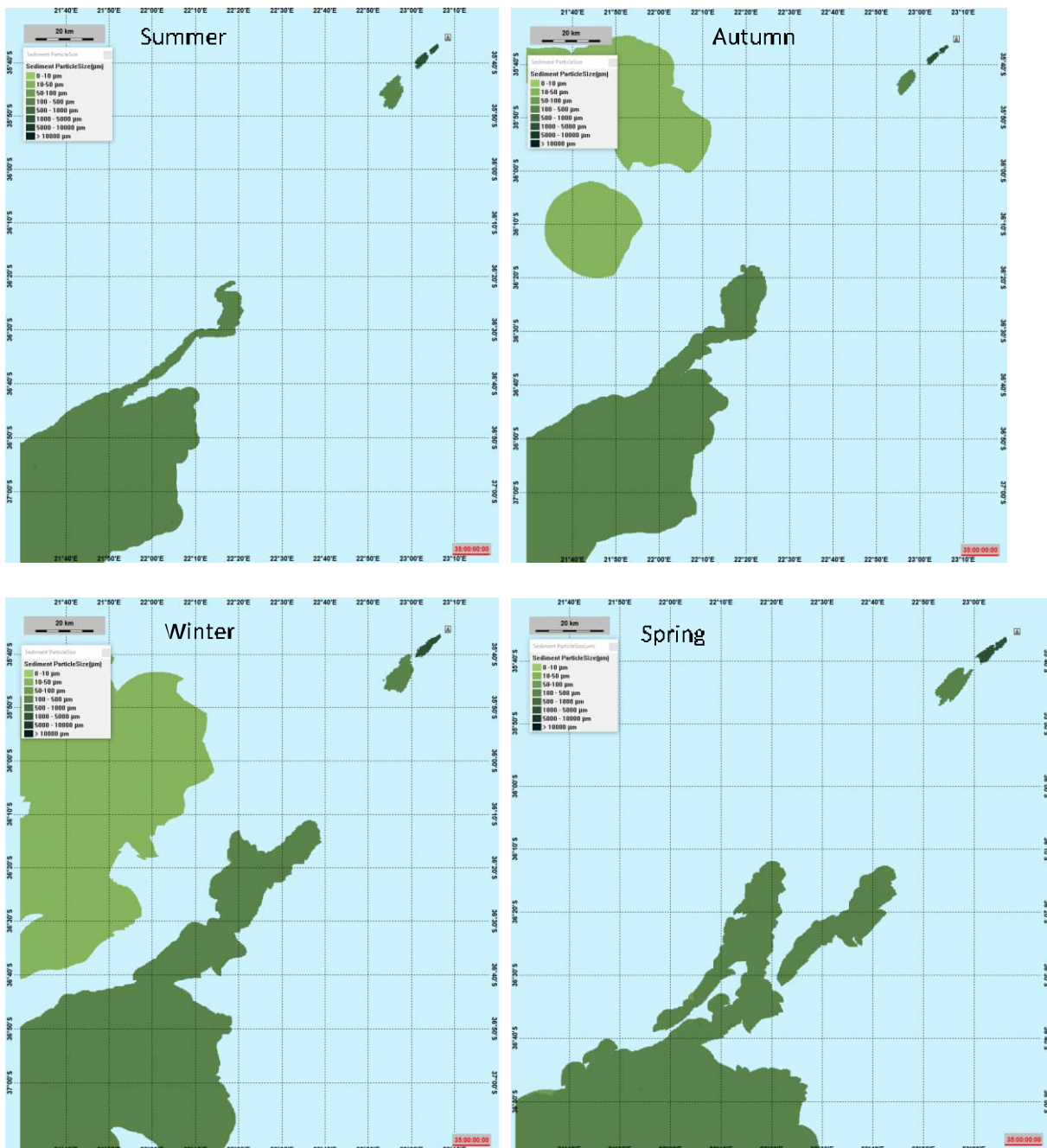
Figure 9.61 Calculation of median grain size deposited at the sea floor after completion of the discharge from rig for discharge location 5 for all four seasons.
