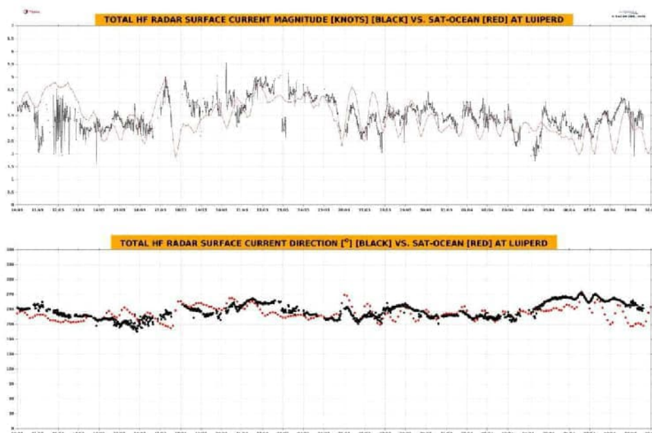
Figure 4: Surface currents time-series from SAT-OCEAN (model) vs HF Radar (observations) for 30 days.
