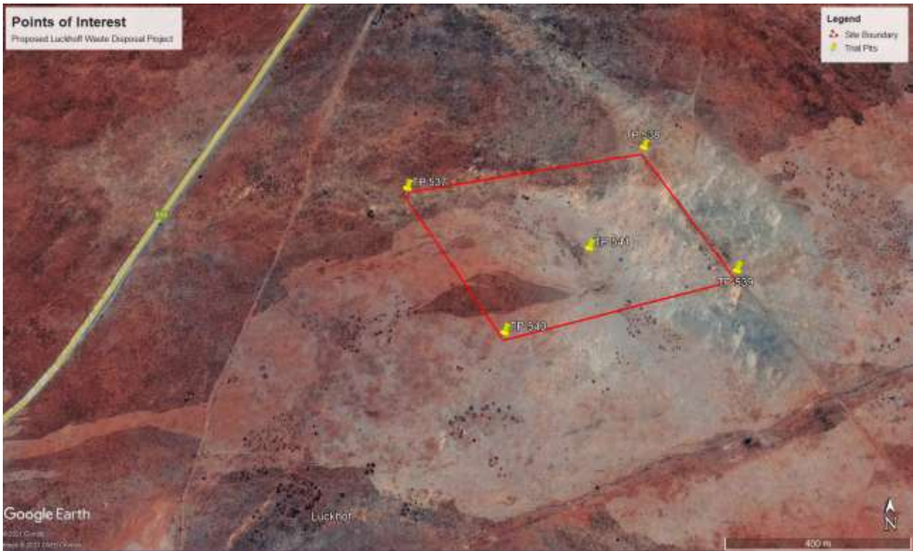
Figure 2: Approximate Site Boundary with 5 trial pits positions
