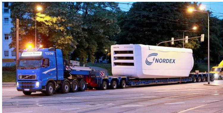
Figure 7.3 Example of Nacelle Transport ( Recharge News )
