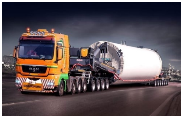
Figure 7.1 Example of Steel Tower Sections Transport (Nooteboom)
