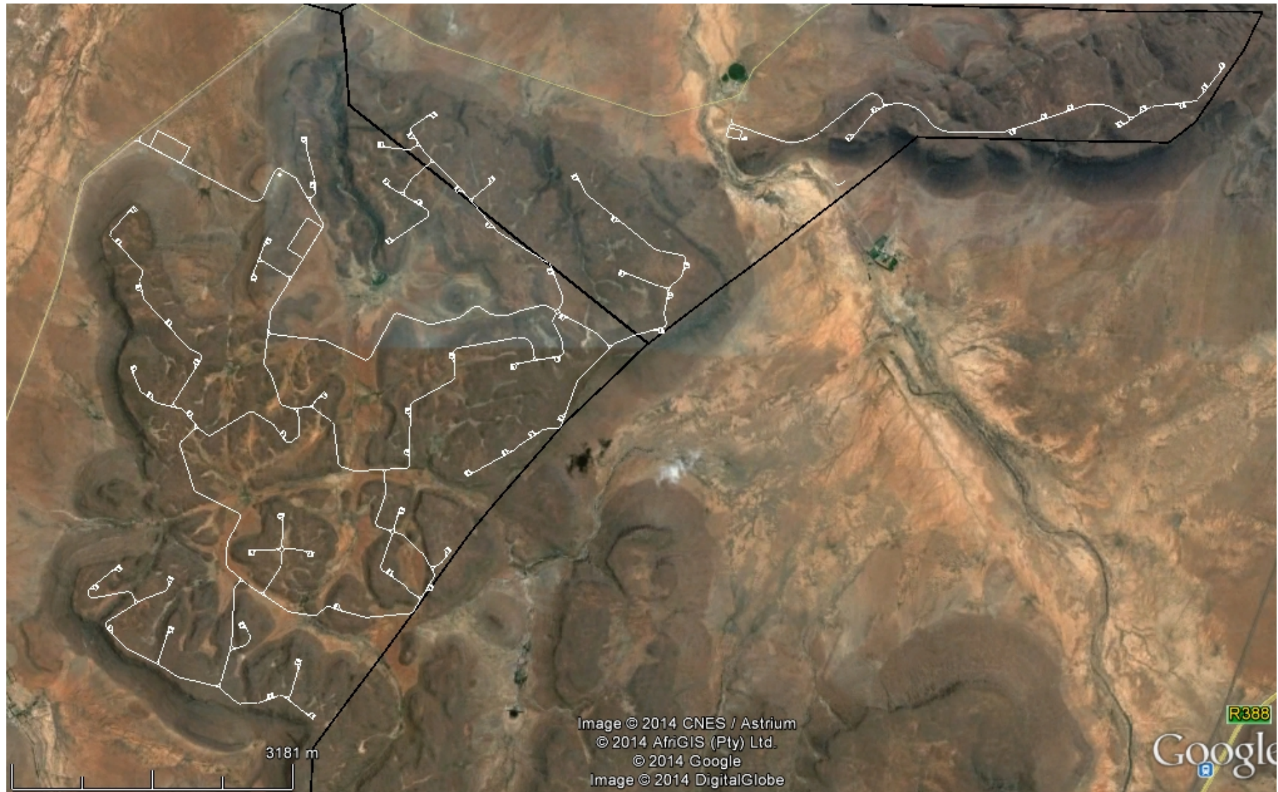
Figure 1: Map overview of the proposed developmental footprint (white) of the Maanhaarberg WEF. Development site boundaries in black.
