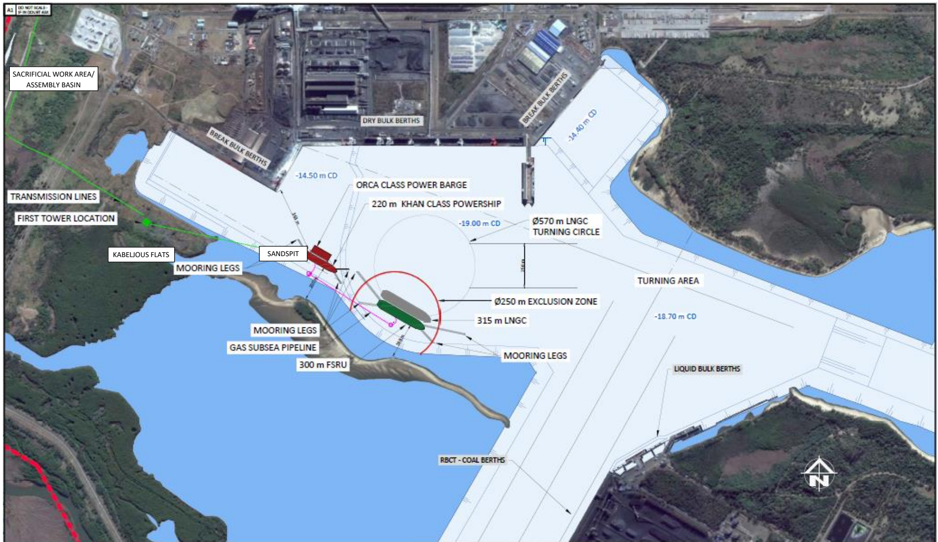
Figure 2. Alternative layout 2 of the proposed Gas to Power components within the Port of Richards Bay
