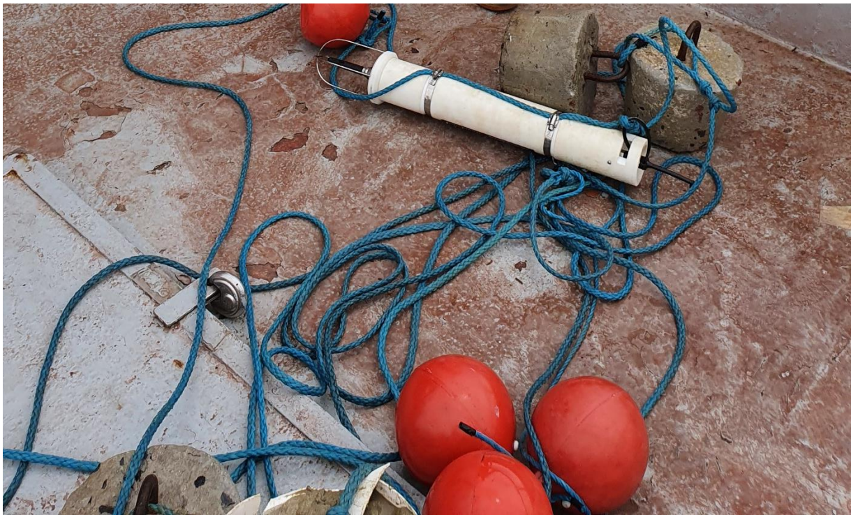
Figure 5-9 – Static monitor, ropes, buoys and weights on deck
