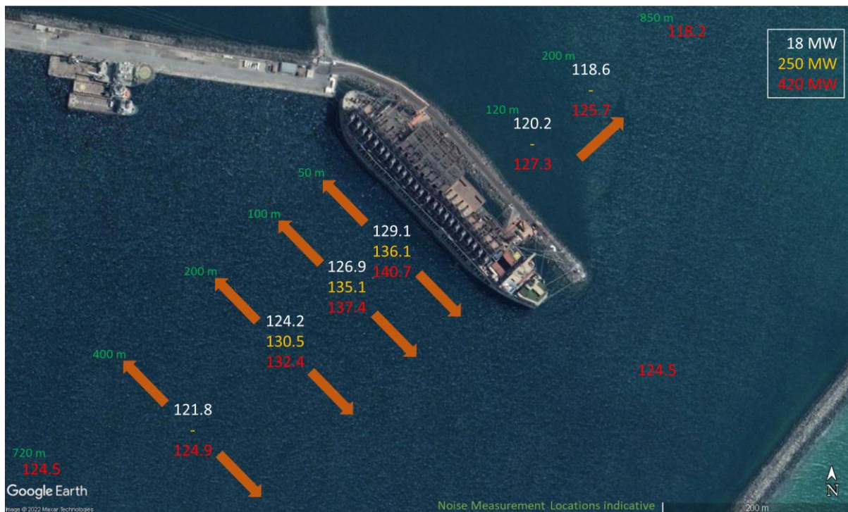
Figure 4-3 – Average of underwater noise measurements sampled along lines at the Osman Khan Powership in Ghana under various operating conditions
