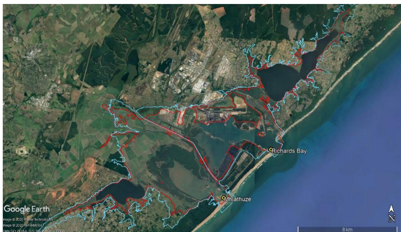
Figure 7. Estuarine functional zone of the uMhlathuze/Richards Bay estuarine system, as delineated by the 5 m contour in red, and 10 m contour in blue (Image source: Google Earth; National Estuaries layer CSIR 2018a)
