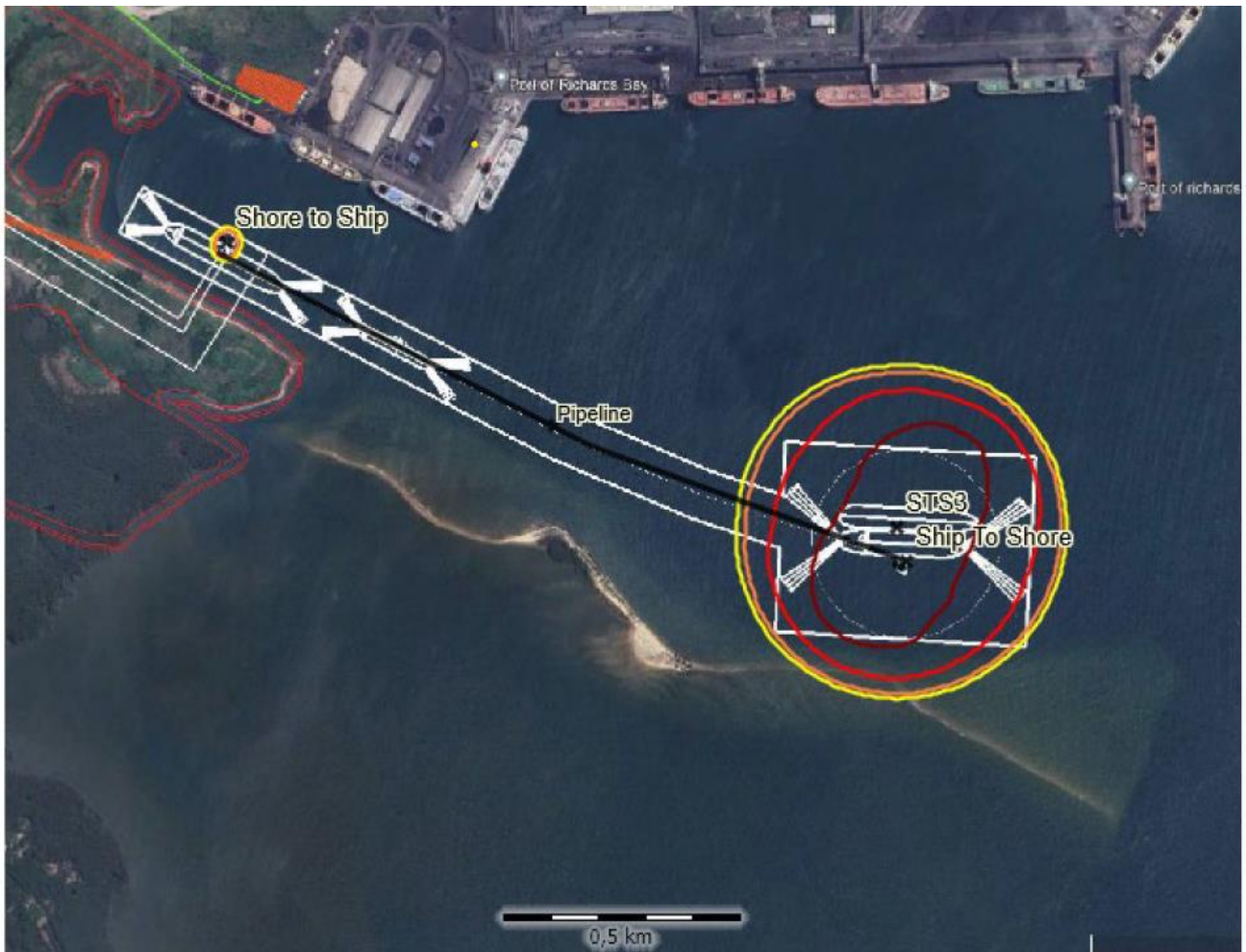
Figure 31. Individual risk horizons calculated for the Gas to Power project: 1:10 000 (red), 1:100 000 (orange), 1:1000 000 (yellow) and 1: 30 000 000 (green)
