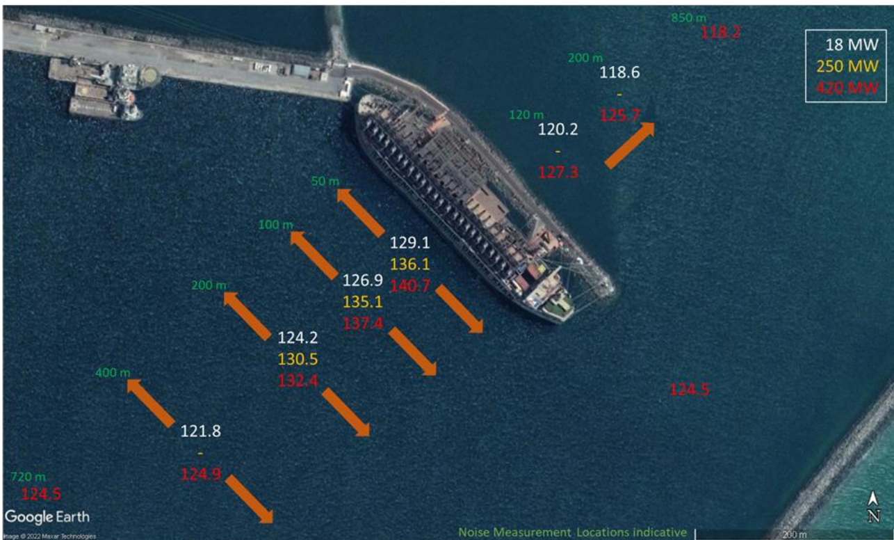
Figure 27: Average of underwater noise measurements sampled along lines at the Osman Khan Powership in Ghana under various operating conditions. All measurements are logarithmic averaged decibel SPLRMS re 1 \mu Pa. This shows the underwater noise levels averaged over each line, recorded when the ship was producing power with one engine (approximately 18 MW), 14 engines (250 MW) and 23 engines (420 MW) (Subacoustech Environmental Report No. P292R1001, 2022).
