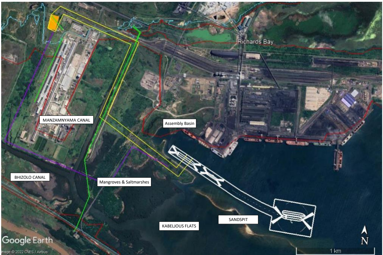
Figure 4. Location of the proposed Gas to Power components within the Port of Richards Bay, indicating the corridor of the alternative 1 transmission line route (yellow), the alternative 2 route (purple), switching station (orange polygon) existing Municipal transmission line (green), relative to the 5 m (red) and 10 m estuarine functional zone (blue) boundaries (Image source: Google Earth, 2022)
