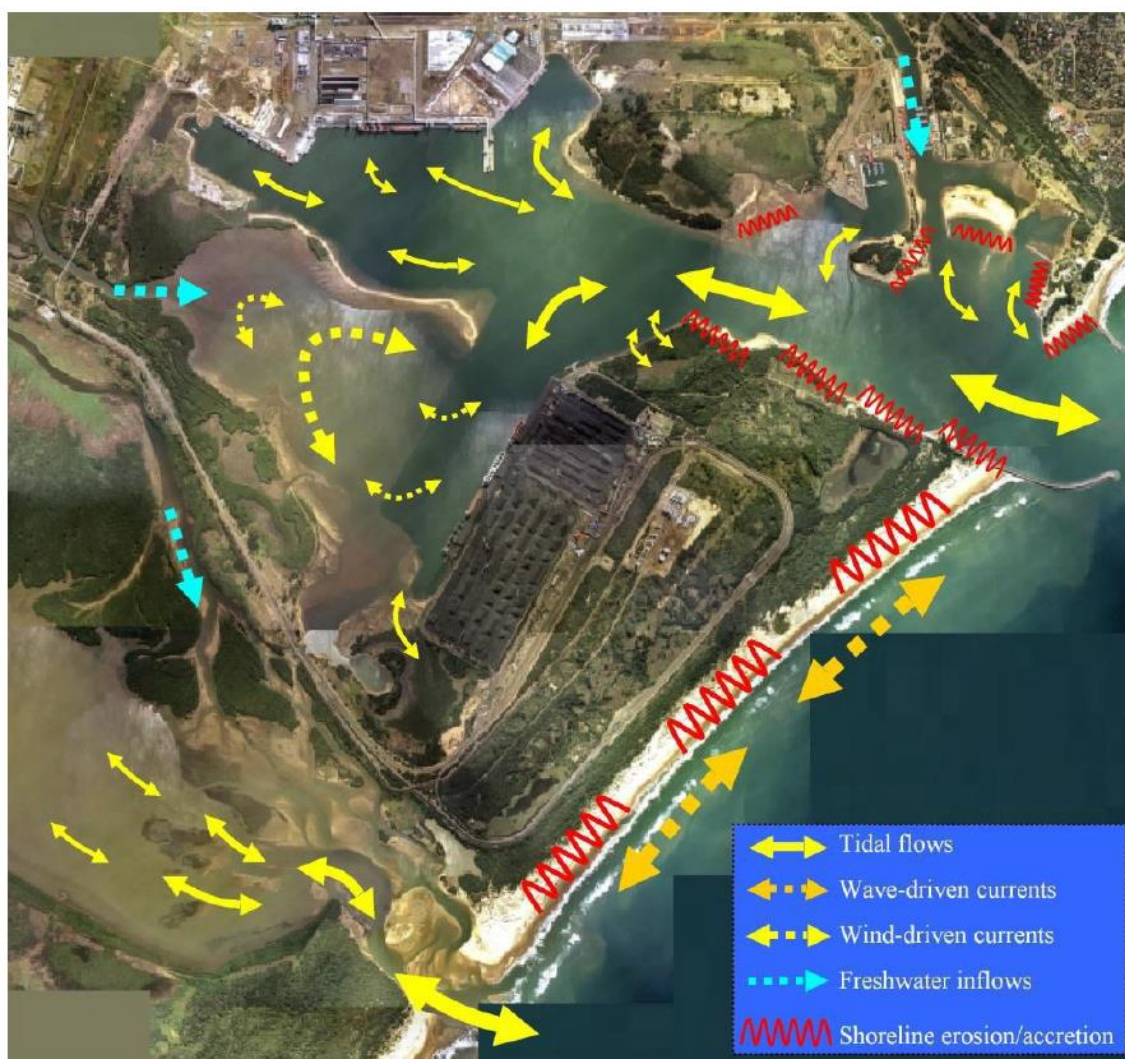
Figure 8. Schematic of major hydrodynamic processes within the Port of Richards Bay and adjacent coastline (modified from van Ballegooyen et al. 2015). The red rectangle demarcates the proposed Project development area.
