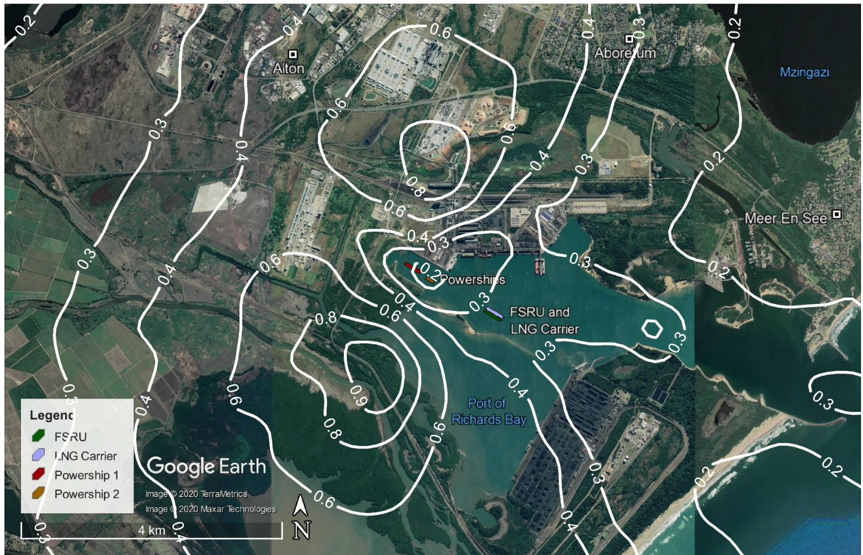
Figure 13: Predicted 99 th percentile 1-hour SO 2 concentrations in µg/m 3 resulting from emissions from the Karpowership Project
