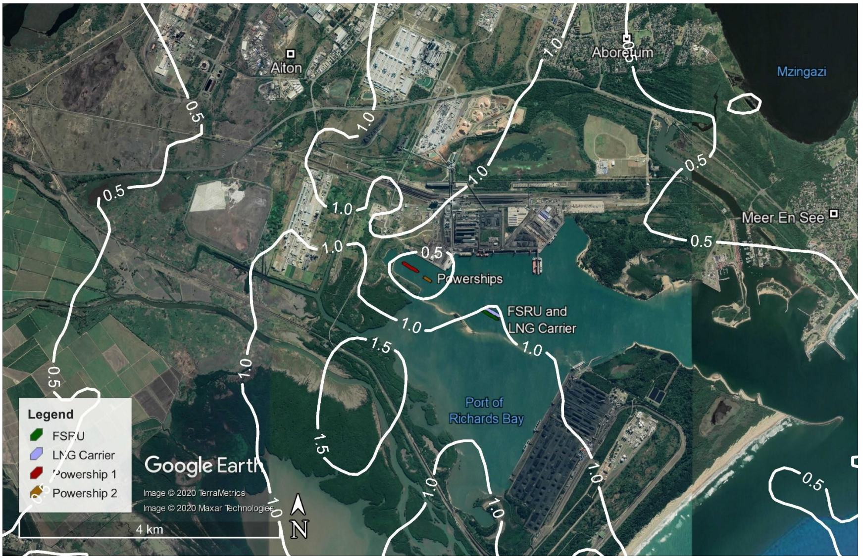
Figure 17: Predicted 99 th percentile of the 24-hour PM 10 concentrations in µg/m 3 resulting from emissions from the Karpowership Project
