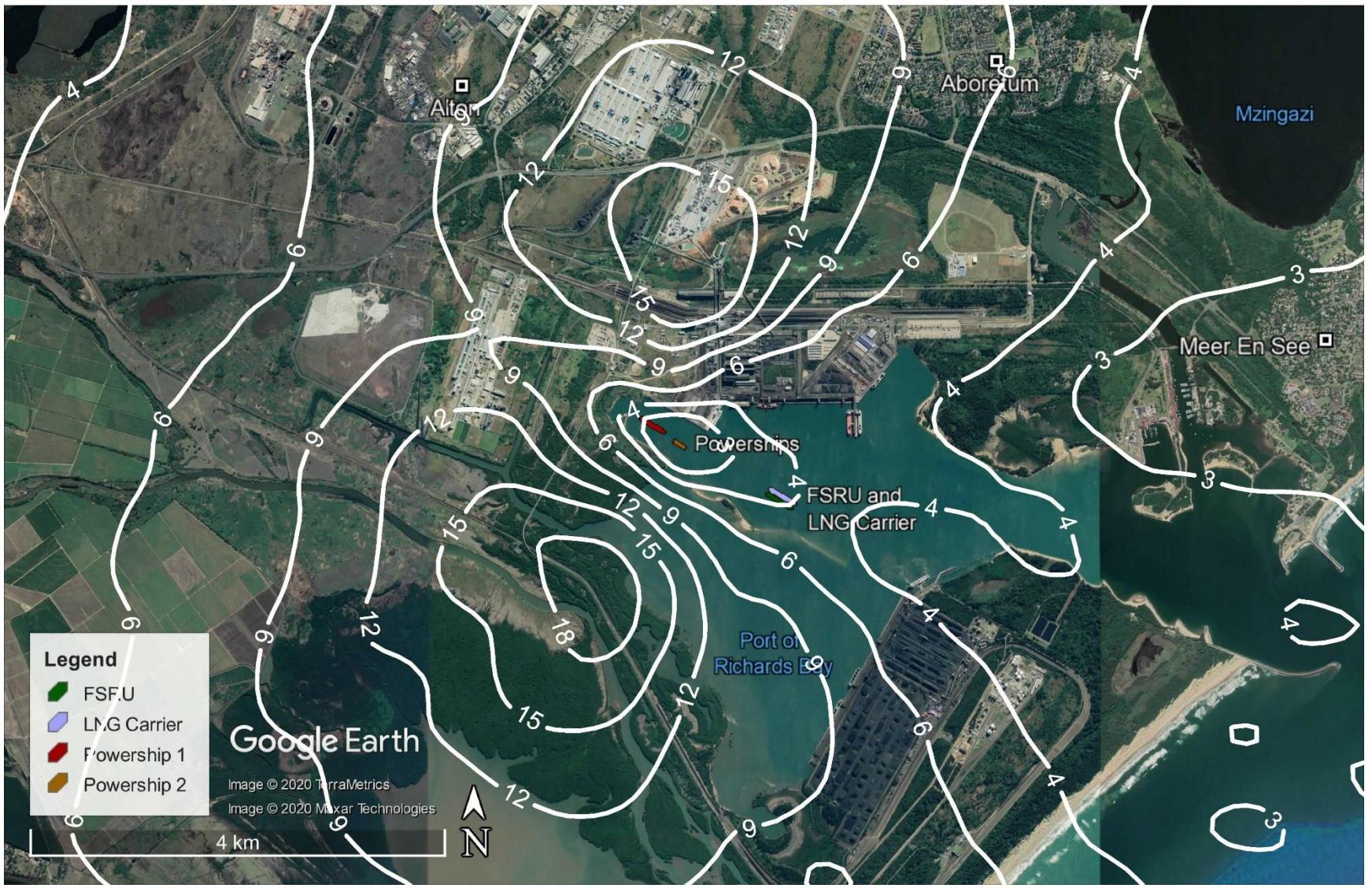
Figure 15: Predicted 99 th percentile 1-hour NO 2 concentrations in µg/m 3 resulting from emissions from the Karpowership Project
