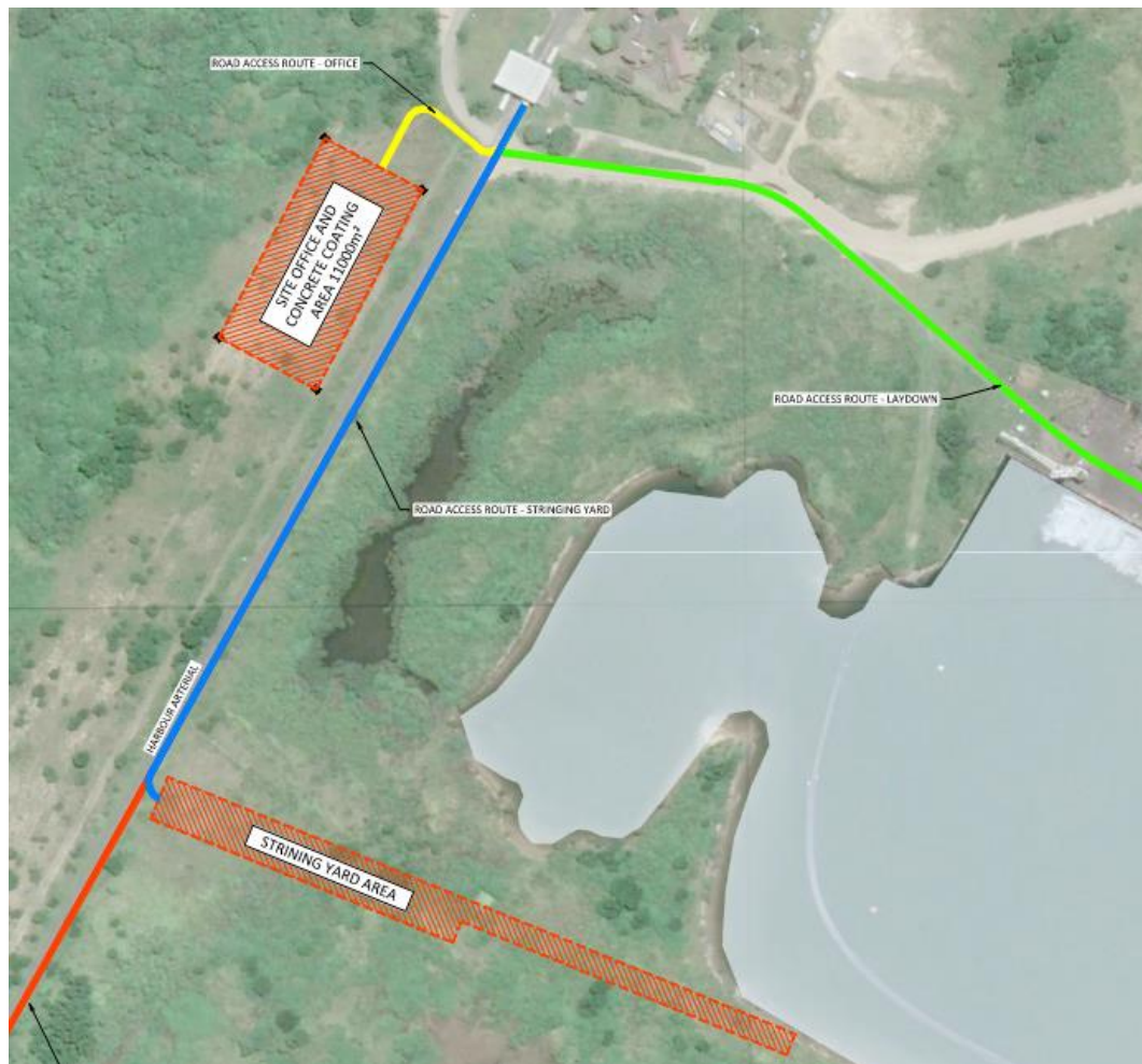
Figure 3: Stringing Yard (Source: PRDW S2117-07-DR-GA-202-S1-A)
