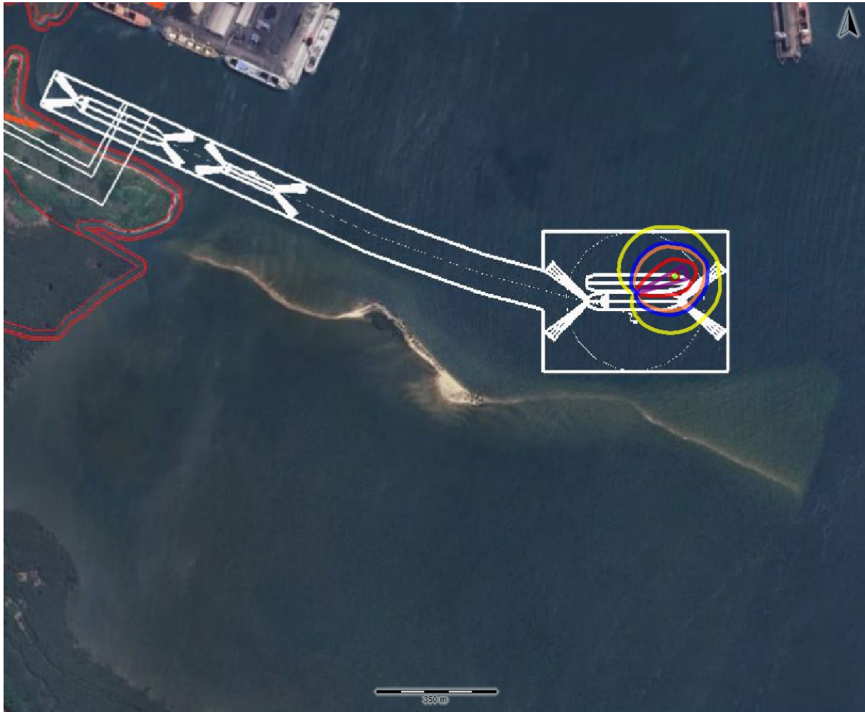
Typical 1-inch Jet Fire at the STS Transfer Hose
