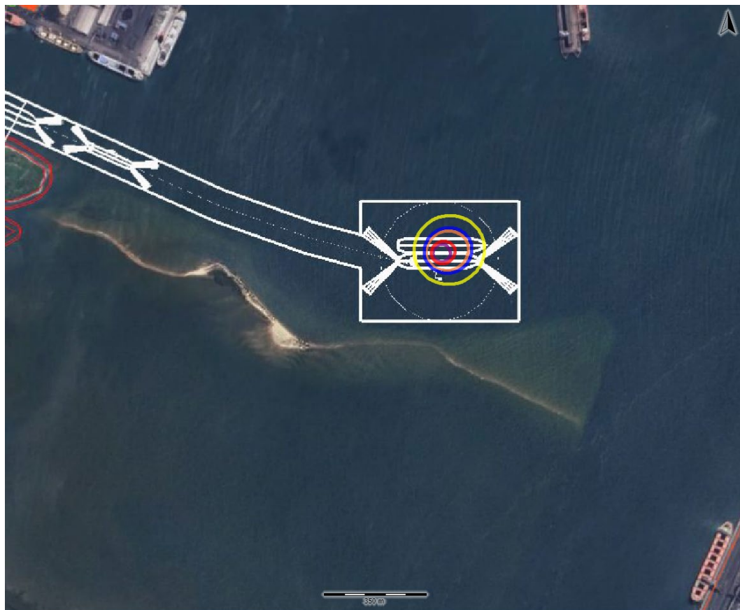
Pool Fire as the Result of a Hose Rupture
