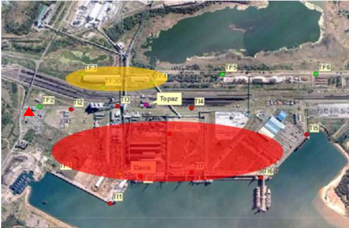
Figure 11: Broad analysis of areas of high dust impact for Transnet Terminal dust monitoring network (WSP, 2008, 2012). Includes approximate location of Bayside SO 2 monitoring site (red triangle) (RBCAA, 2012).
